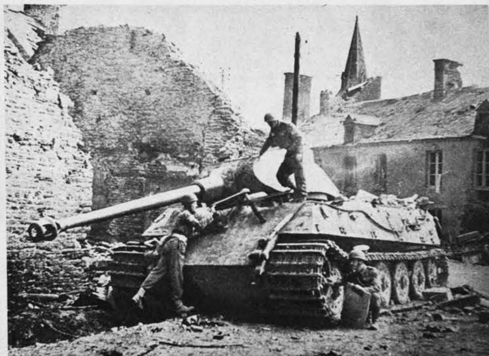
Latest Nazi heavy tank is 67-ton "Pan Tiger" or "Royal Tiger." Bigger than the Tiger (PzKw VI) and just as heavily armed, it is a scaled-up Panther (PzKw V) in appearance.
